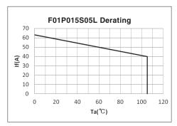
Figure 4: Ip vs Ta for F01P015S05L
