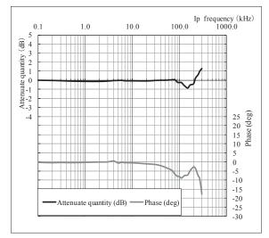
Figure 2: Frequency response curve ex) F01P025S05L
