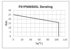
Figure 3 : Ip vs Ta for F01P006S05L
