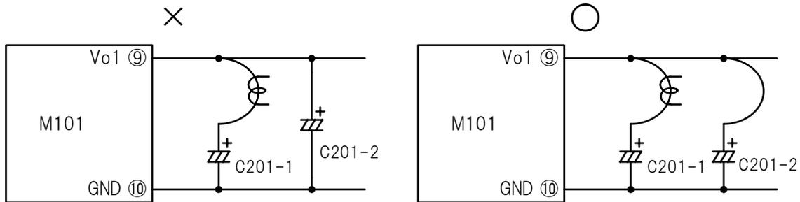
When current measurement leads, etc. are installed Only to the capacitor to be measured, the impedance is unbalanced and accurate measurement is not possible.
