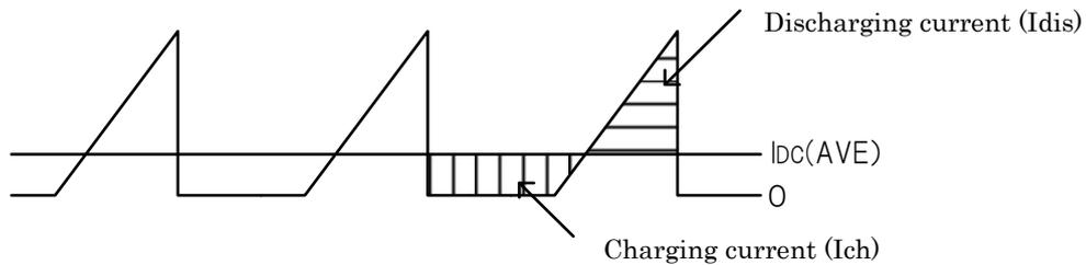
$$I_{ripple} = \sqrt{I_{dis}^2 + I_{ch}^2}$$
