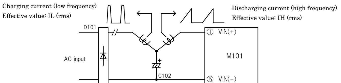
The ripple current ( $I_{120}$ ) frequency corrected to 120Hz is calculated from the following expression:
