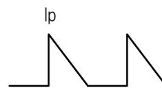
High frequency current also flows in L201 and C202. Check that L201 is not saturated even at  $I_p$ .
