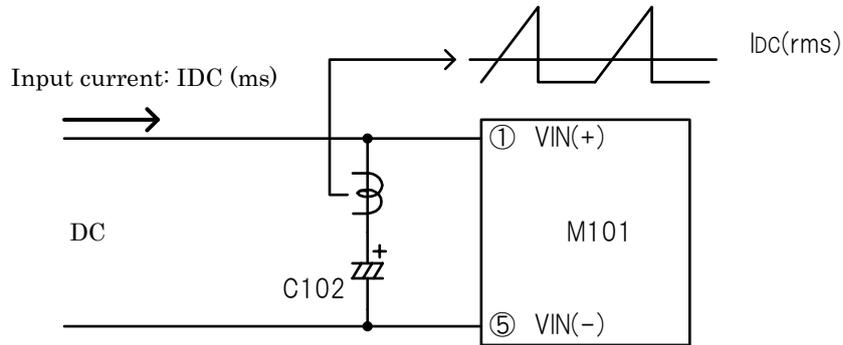
The ripple current of an electrolytic capacitor is a triangle wave high frequency current with the input current (DC current) made the average value. Ripple current is calculated as follows:
